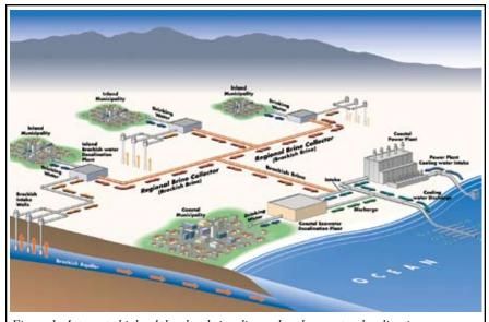
Figure 1. Integrated inland desalter brine disposal and seawater desalination.
